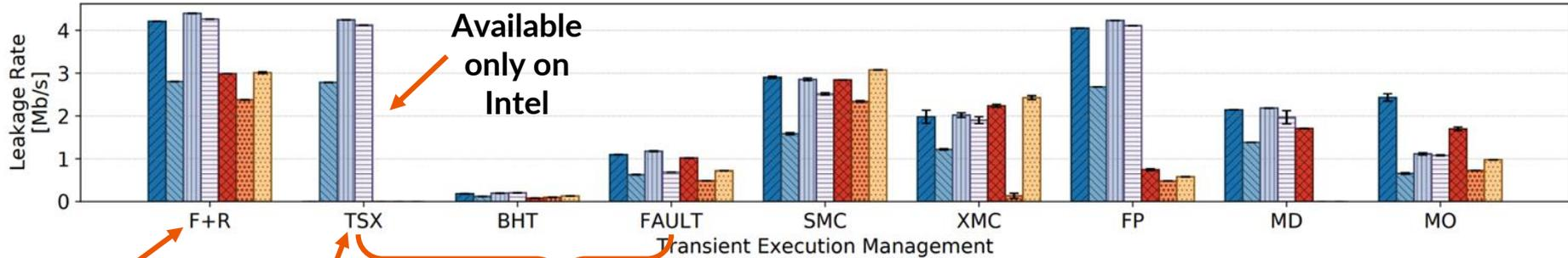
Architectural upper limit leakage rate
